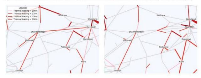
Figure 49: Transmission network needs assessment of the Midlands, 2027 (left) and 2030 (right)
