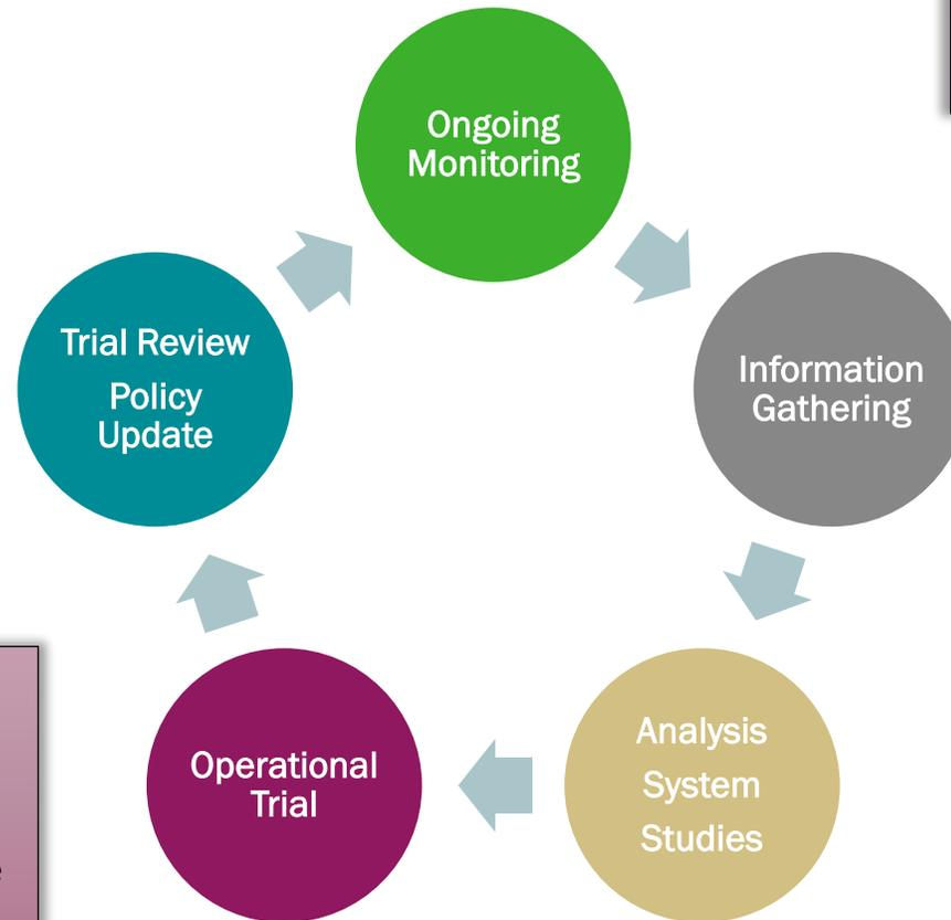
In the Ongoing Monitoring phase, EirGrid and SONI engineers monitor the system parameters and analyse events and disturbances to assess system performance and generator compliance relative to operational policy parameters and metrics.
