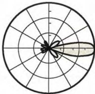
Fig. 6: Typical Narrow Beam-Width Aerial Radiation Pattern
