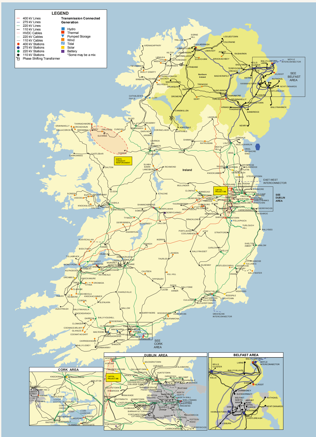
Figure A-2: Planned transmission system 400 kV, 275 kV and 110 kV, December 2031
