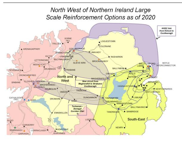
Figure 6-2 North West of NI Large Scale reinforcement - potential options
