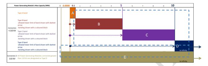
Figure 2 - Limits for thresholds for type B, C and D power-generating modules
