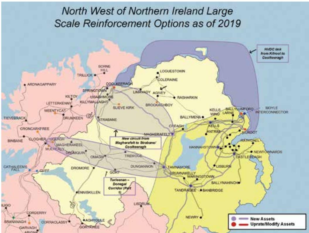
Figure 6-2 North West of NI Large Scale reinforcement – potential options
