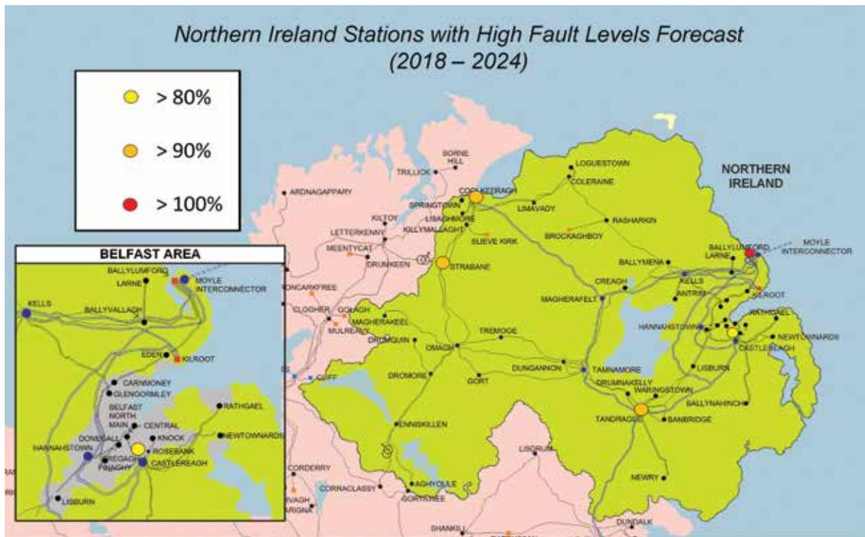
**Figure 5-1 Stations with forecast high fault levels, 2018 – 2024 (from TYTFS 2018)**
