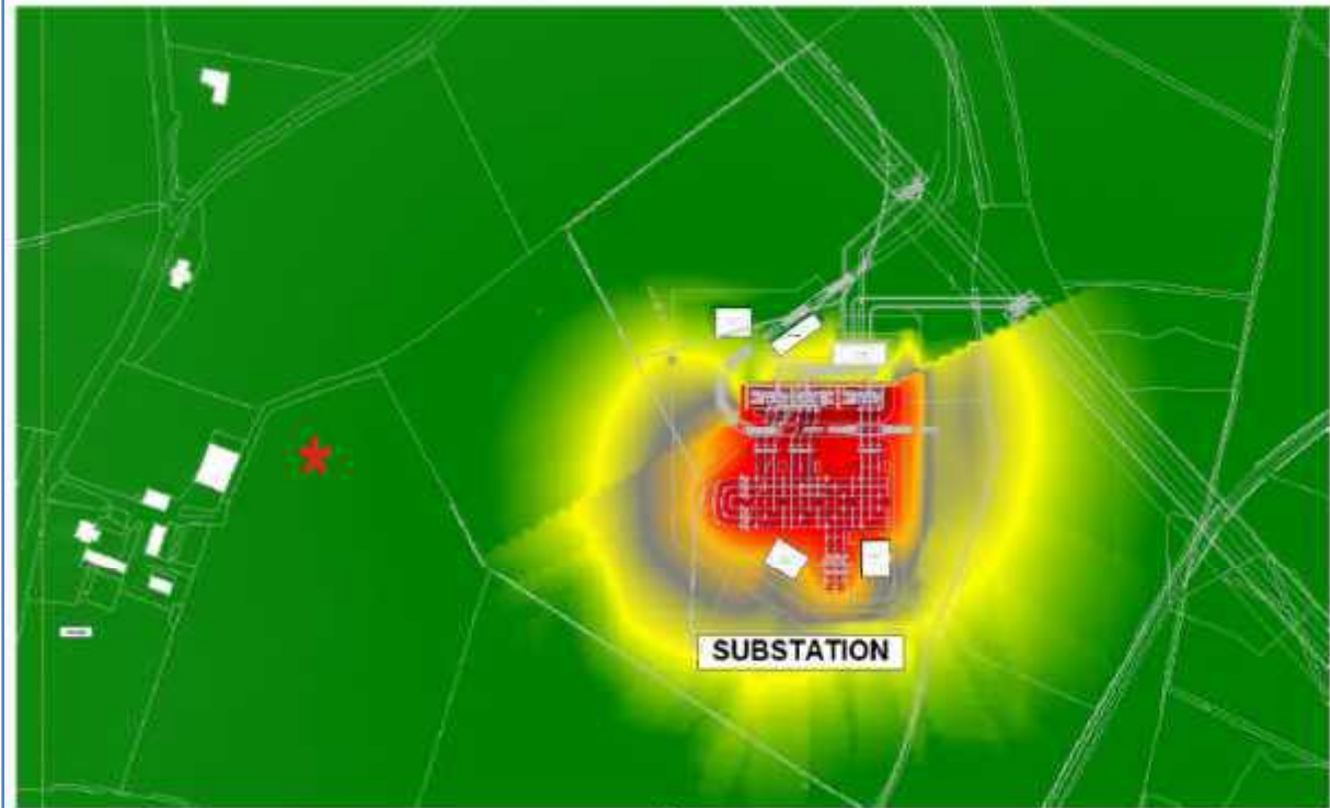
Illustration 11.1: Substation Noise prediction model screenshot (not to scale)
