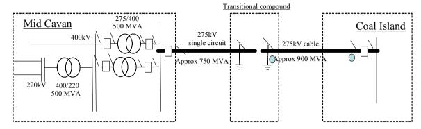
Figure A.1: Initial Phase of 275kV single circuit
