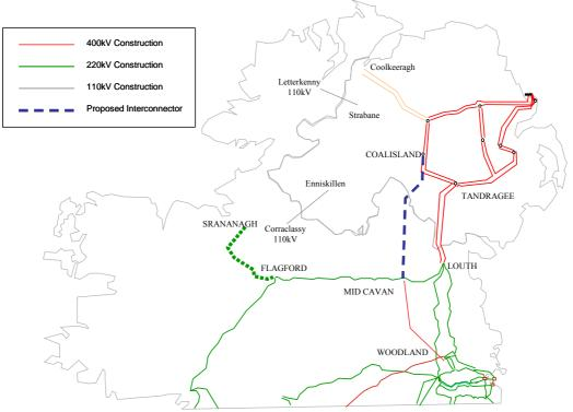
Figure 1: Network Schematic showing Proposed Interconnector
