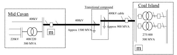
Figure A.3: initial phase of 400kV single circuit – approx 900 MW – used for cost comparison
