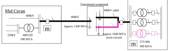
Figure A.4: Final Phase 400kV single circuit – increase to 1500 MW
