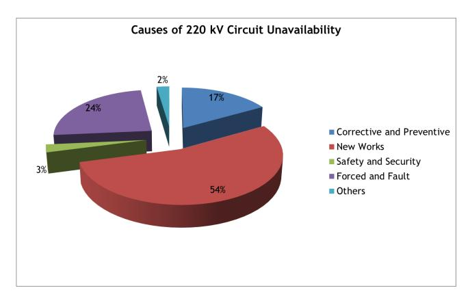
Figure 11: Causes of Unavailability on the 220 kV System in 2023
