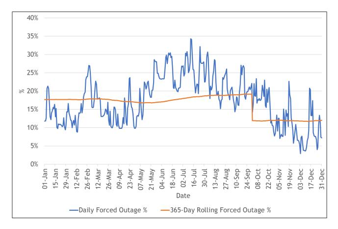
Figure 2: All-Island Dispatchable Conventional Generator (including AGUs) Forced Outage % 2023
