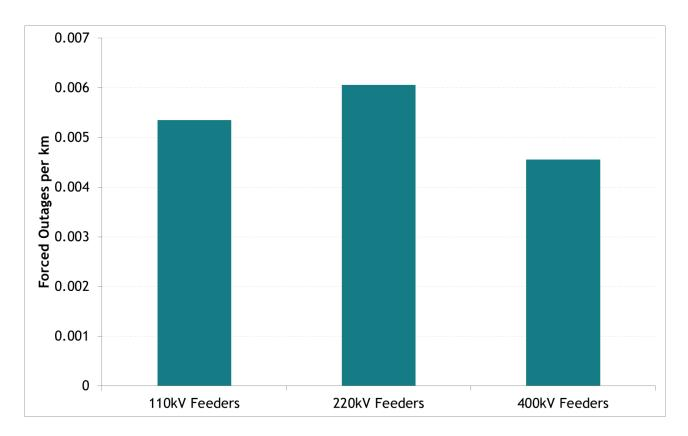
Figure 17: Forced Outages of lines and cables per km in 2023.
