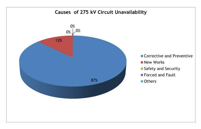
Figure 12: Causes of Unavailability on the 275 kV System in 2023
