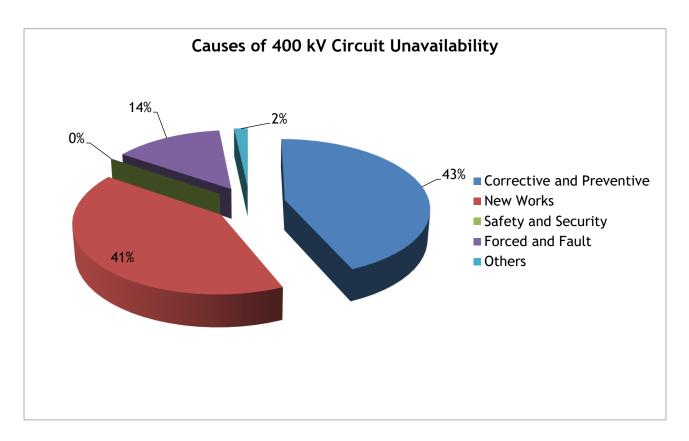
Figure 13: Causes of Unavailability on the 400kV System in 2023
