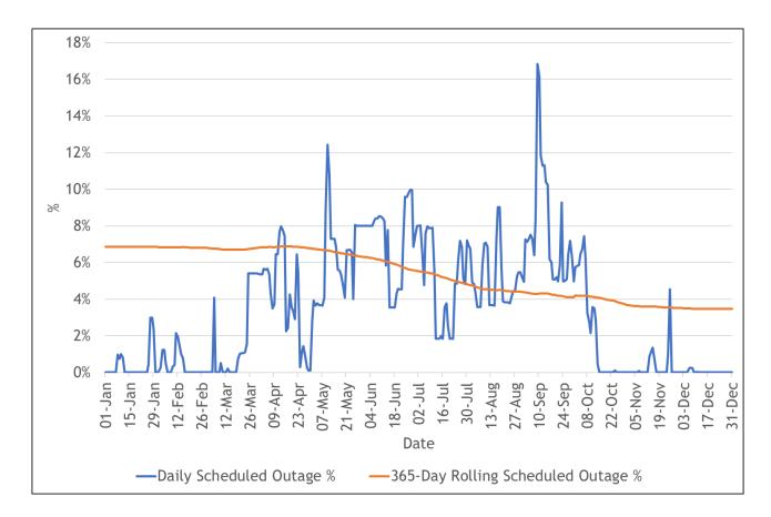
Figure 3: All-Island Dispatchable Conventional Generator (including AGUs) Scheduled Outage Rate 2023
