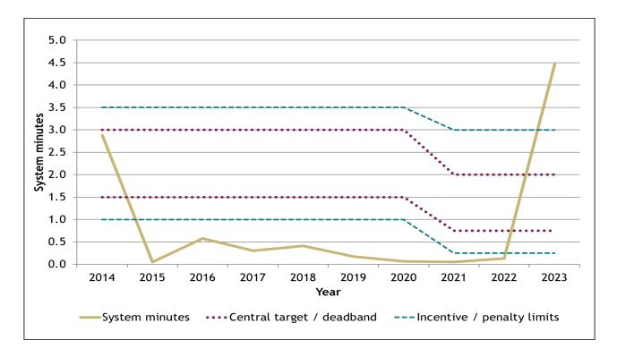
Figure 7: System minutes lost and associated targets: EirGrid 2014-2023
